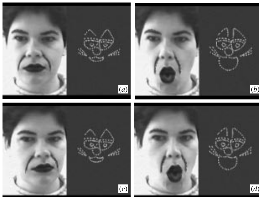
Figure 4. Pose-invariant transmission of facial expression. Separation of non-rigid from rigid motion by SVD is used here to extract the facial expression of an actor. The extracted expression is displayed on this cat caricature in a fixed pose, and can be seen to be independent of the pose of the actor's head.
